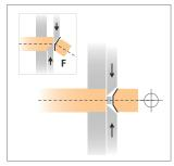
The blades are arranged in one plane and therefore do not generate any transverse forces during cutting and stripping.
