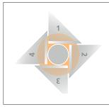
Because of the 4 blades (large contact surface), even thin and strongly adhering insulations can be removed.
