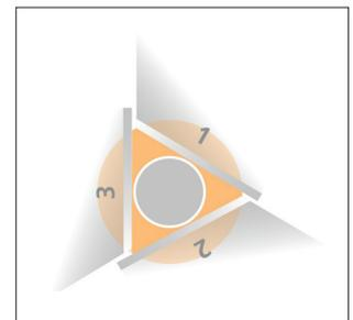
Due to the large contact surface, the 3 knives provide an advantage over a two-knife stripping head when stripping strongly adhering insulations.
