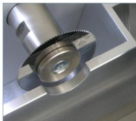
Carbide saw blade for long life and precise sawing.
