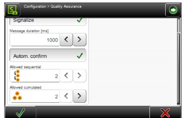
As soon as one of the two counters is reached and the defective piece has been rejected, the machine stops and error message 5955 appears with the following informations:
