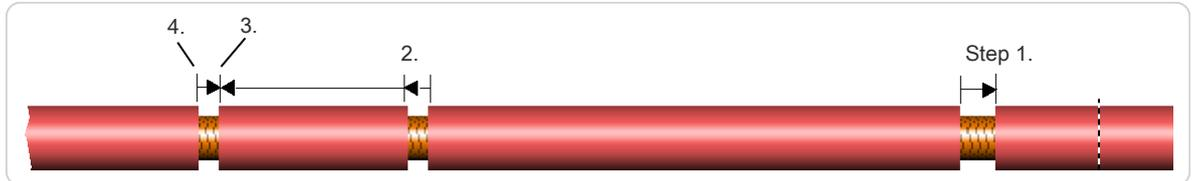
Fig. 17: For example, pull-off in several steps
