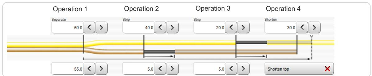
**Operation 1:** Defines the separation of the wires:
