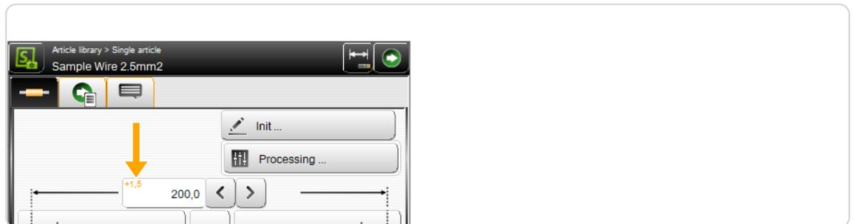
If the correction mode is on, the user opens directly the numeric touch-keyboard by touching **[ENTER CORRECTION VALUE]** where the effective measured length can be entered.
