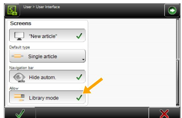
The "Library mode" provides additionally the application type called "User defined". This way also multi-step stripping can be performed.
