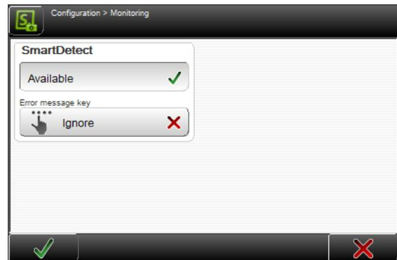
If a SmartDetect contact occurs during production, warning 5955 appears with a detailed description of the contact and recommendations for further action to resolve the problem.
