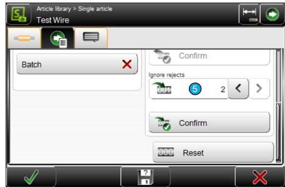
3.▶ A total of 8 pieces were produced, 2 more than planned. This causes the machine to automatically start another production cycle. Therefore, the “Produced” field **2** shows the difference between the actual number of pieces produced (8 in total) and the planned number **1** (here 6), i.e. 2. In the “Remaining” field **5** the difference between the planned number (here 6) and the number in the “Produced” field (here 2) appears, i.e. 4. This limitation is known.
